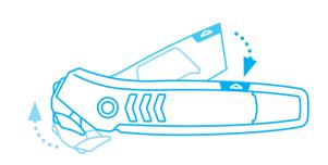
Push the blade magazine **back into the** handle to lock the blade head in place.
