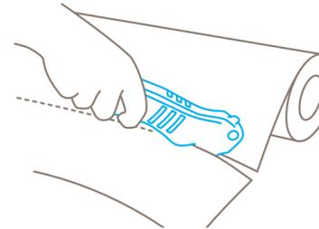
When cutting film and paper, ensure the material to be cut is under **tension**.
